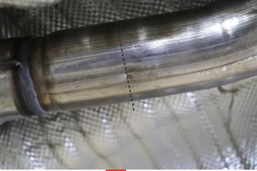
To make it easier to cut the exhaust we reccomend remoiving it from the car. Find the indent just before the resonator to mark out the cutting line. Cut along the line and de-bur the edges. Re-fit the original GPF and fit the Scorpion GPF-back following the line diagram on the first page.
